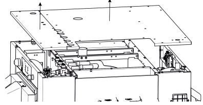
**STEP 2** : Using the drilling template, drill the small cap with 4 holes provided for installing the connectivity card (Fig.2)
