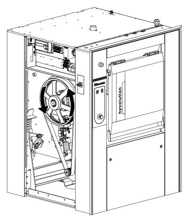
· Check the direction of rotation of the circulating pump and of the draught accelerator gas heating.
