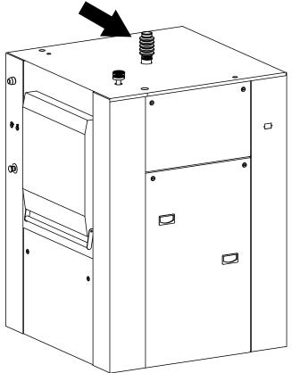
It is important that the machine is put at atmospheric pressure as the levelling of water depends on it. Alternative 1:
