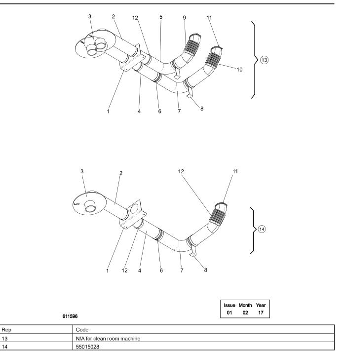
Replace the casings after taking care to remove the pre-cut of the left casing to allow the pass of the rubber hose.
