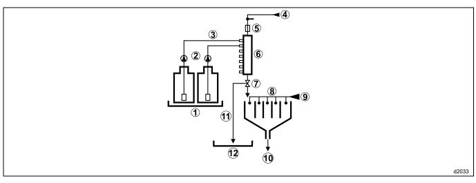
Multi-inlet dose controller with a compulsory rinsing device.
