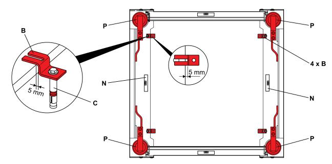
Weighing equipment: P Water level: N Fixing dowels: C Flange safety locks: B
